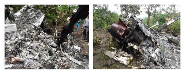
The main rotor transmission, main drive shaft, mast, main rotor hub, blades and stabilizer bar were all found attached together lying in farther most point from the tail boom.
