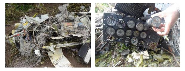
• The floor panel of the cabin was completely uprooted with all the passenger seats flung on the ground either in burnt or completely broken condition.
